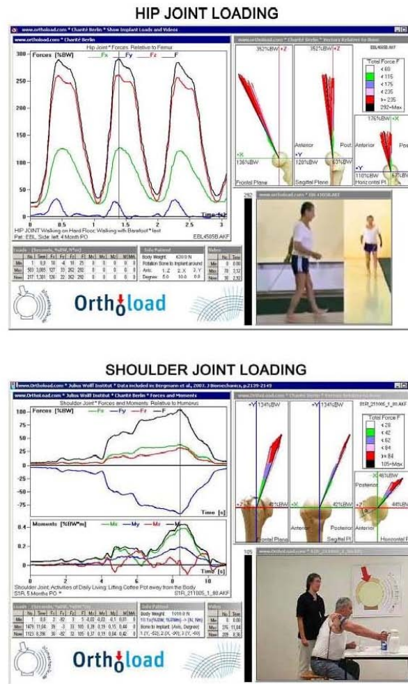
Figure 2. Examples of loading profiles measured in vivo using telemetric implants. TOP: loading in the hip joint during gait (3 steps). BOTTOM: loading in the shoulder while lifting a coffee cup (reproduced from http://www.orthoload.com/ ).
